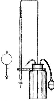
carrying a clamp for the burette. The collar and clamp are made of two strips of brass bent as shown in the sketch, which are soldered or riveted together at s. The ends are turned outward, and fitted with thumb-screws, to allow the circles to be clamped firmly about the bottle neck and the burette.
